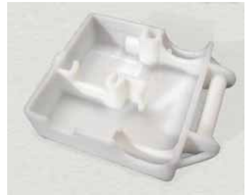
Figure 2: Battery box bottom from Dimension SST
